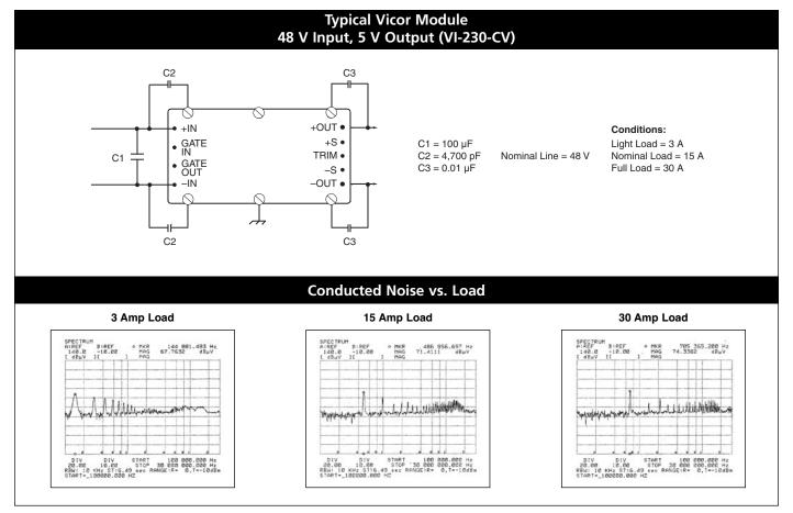
Figure 9–1 — Conducted input noise, no additional filtering
